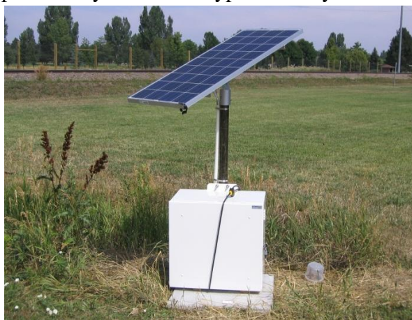
Figure 2.1: A Current Solar-Powered Air Sampler System
